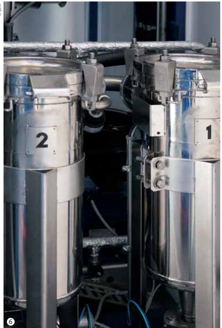
Figure 6: Tanks for collecting the distilled product.
