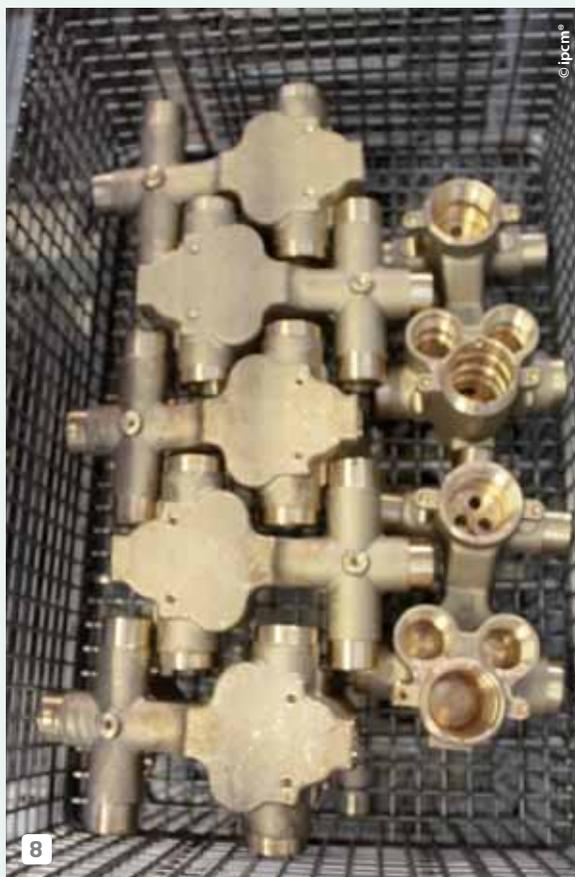
**8** Tap components positioned in the basket before washing: special frames are being studied to facilitate washing complex components that are positioned.
