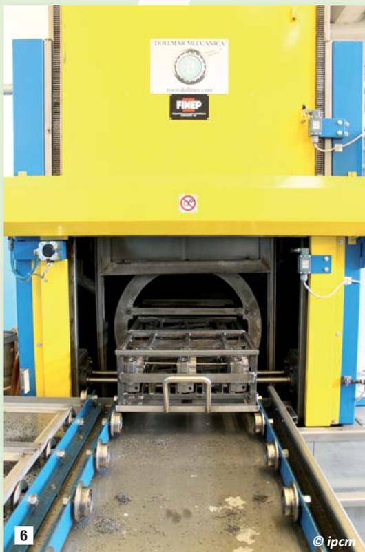
**6** A detail of Dollmar Meccanica's plant: A frame entering the treatment chamber.
