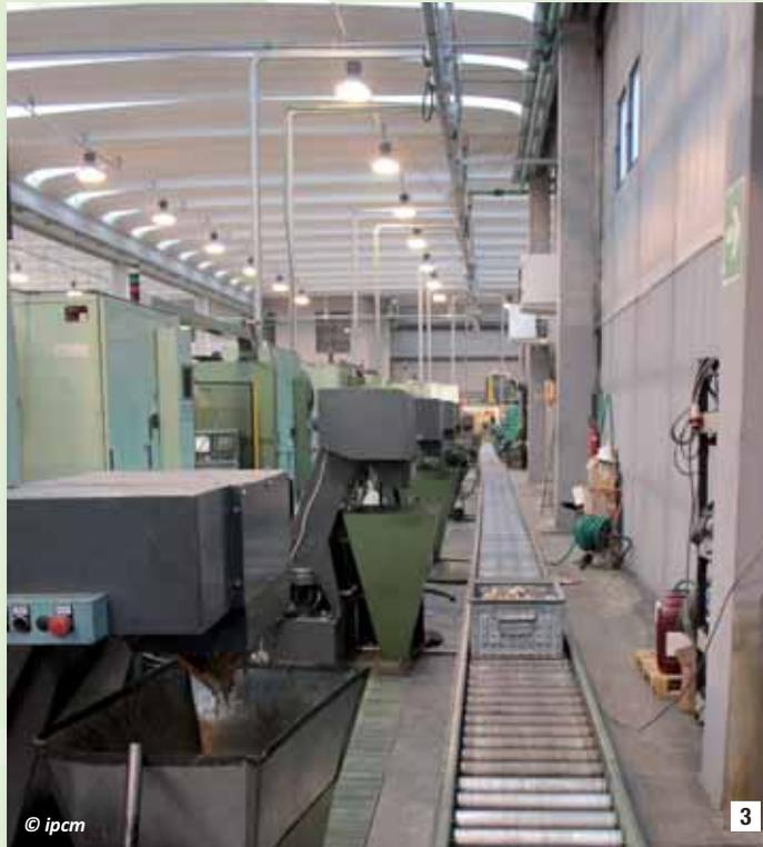
**3** The roller conveyor leads the boxes to the washing station by gravity. At the side of the conveyor, you can see the hoppers that collect the chips exiting the machines in order to recover them.
