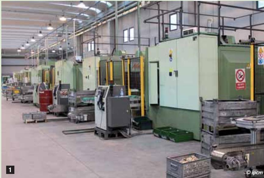
**1** **The 9 robotic stations in the processing area of the plant: Each machining centre is equipped with one or two spindles and with tool changers located above the machine.**
