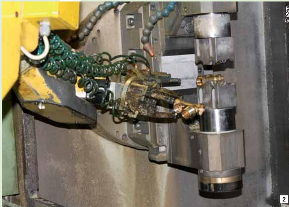
**2** A detail of a robotic arm: The workpiece is placed between the clamps of the machine in order to be processed.
